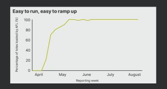
In little over a month, 100% of totes at the ICA CFC in Brunna were processed using the AFL machines, removing the need for labour to complete this task. The chart above highlights the actual percentage of totes processed using AFL at the Brunna CFC.
