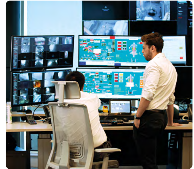
Supervisors Jimmy Ip Lam (left) and Cristobal Ortiz at our Integrated Remote Operation Centre (IROC) in Santiago, Chile, which enables operation at Los Bronces copper mine, 67 km away, to be controlled in an integrated way, and in real time.
