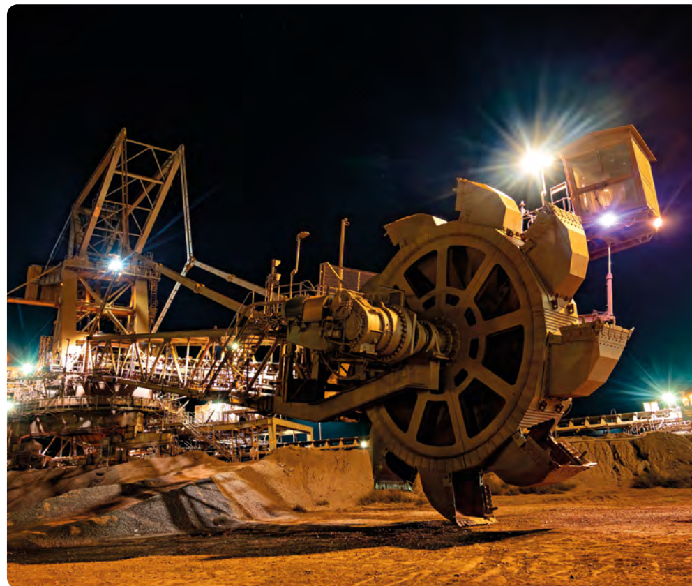
At Kolomela, this bucket wheel excavator and stacker reclaimer work in combination 24/7 to reclaim iron ore and then stack it in bulk quantities.
