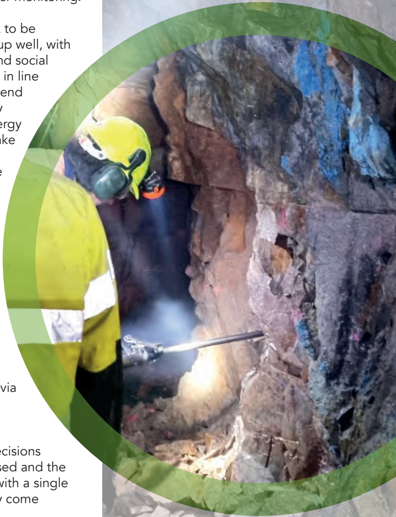
Blast-hole drilling for bulk sample collection at Taronga
