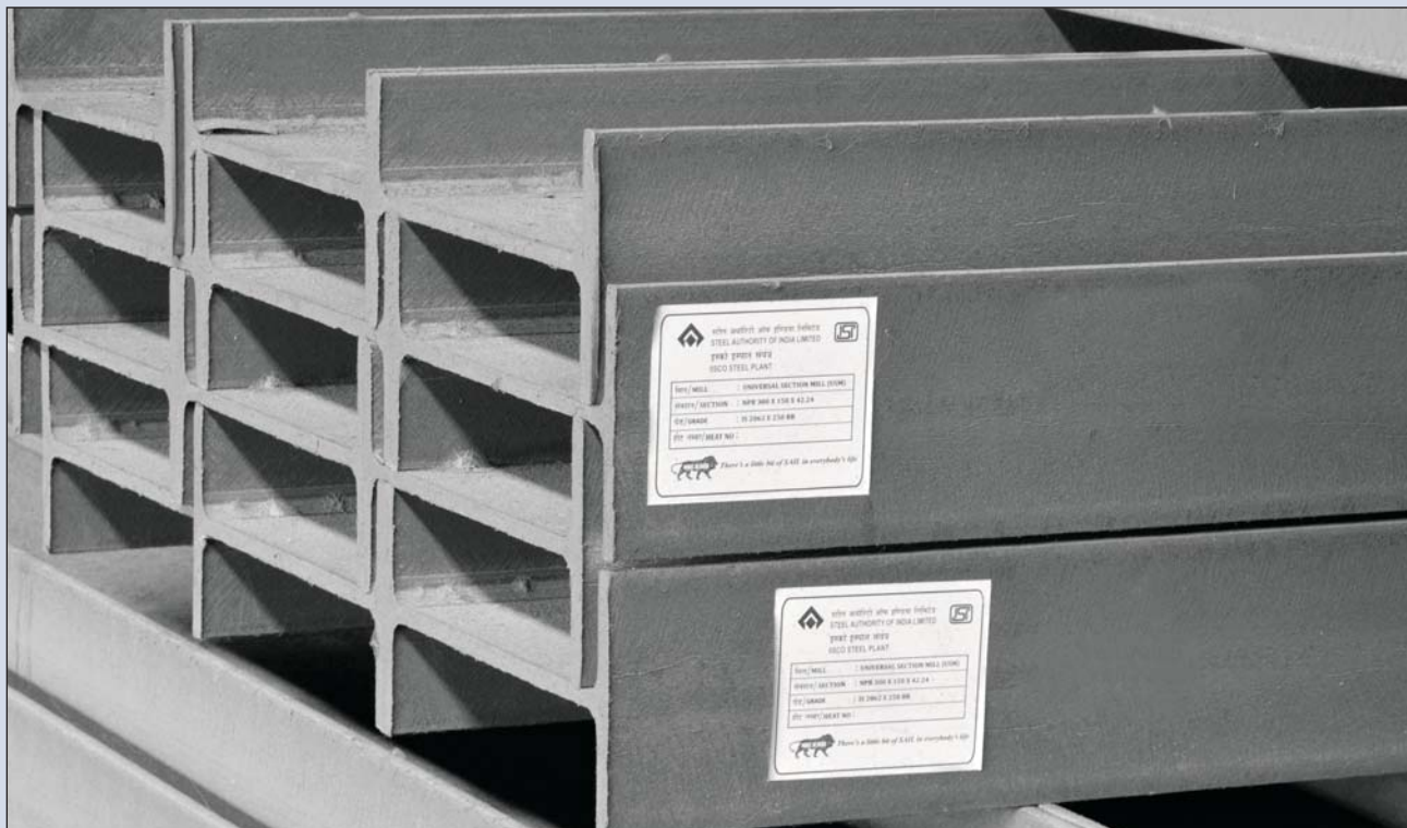
Narrow Parallel Flange Beams manufactured at Universal Section Mill at SAIL's IISCO Steel Plant.
