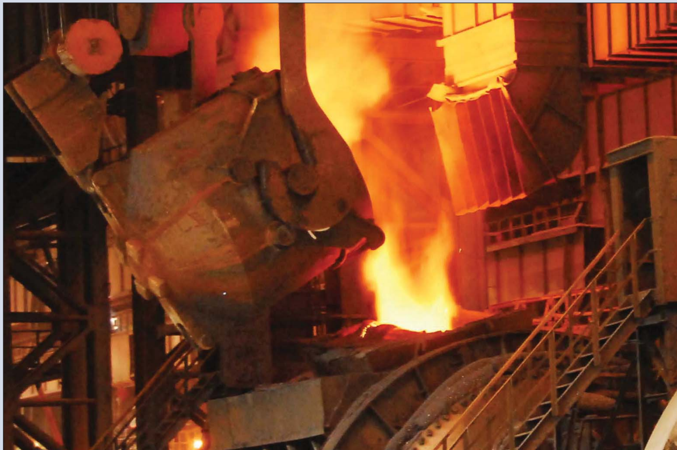
Hot Metal being poured into Mixer of Steel Melting Shop-II at SAIL's Rourkela Steel Plant.
