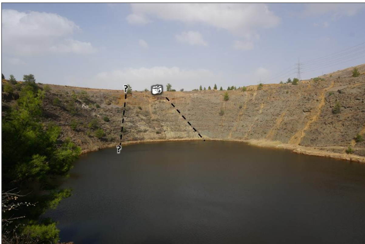
Figure 43 – North Mathiatis – View north from haul road location shown in Figure 44; orebody bounding faults shown. Note strong oxidation and inflow of material from dump to east of pit (Andrew Craig, Nov 2018).
