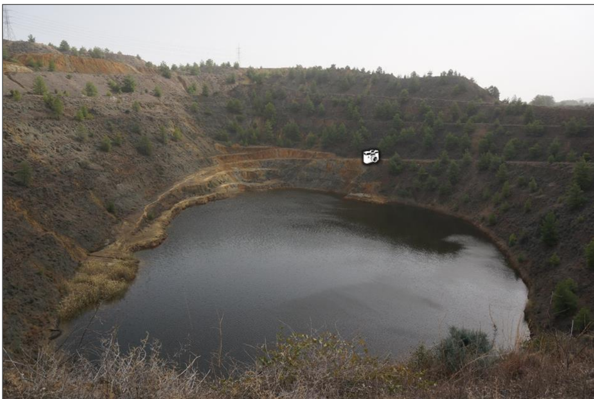
Figure 44 – North Mathiatis – View south from haul road location shown in Figure 43. Note strong oxidation and inflow of material from dump to east of pit. Southern pit floor above waterline exhibits massive and brecciated sulphide mineralisation (Andrew Craig, Nov 2018).
