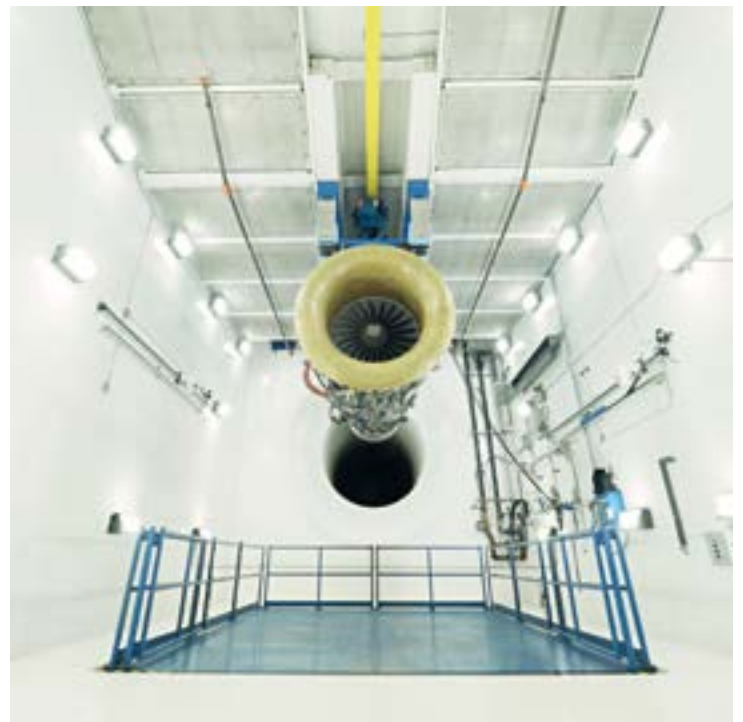
A Rolls Royce Tay engine is set for testing at DAI's new engine test centre facility at Dallas Fort Worth
