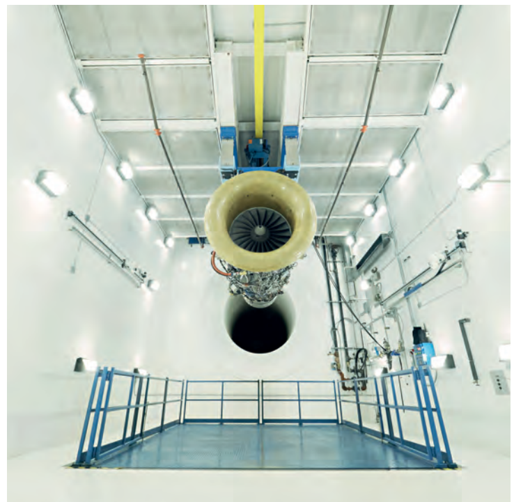
A Rolls Royce Tay engine is set for testing at DAI's new engine test centre facility at Dallas Fort Worth
