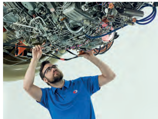
A Dallas Airmotive technician inspects wiring configuration for a Rolls Royce Tay engine preparing for test
