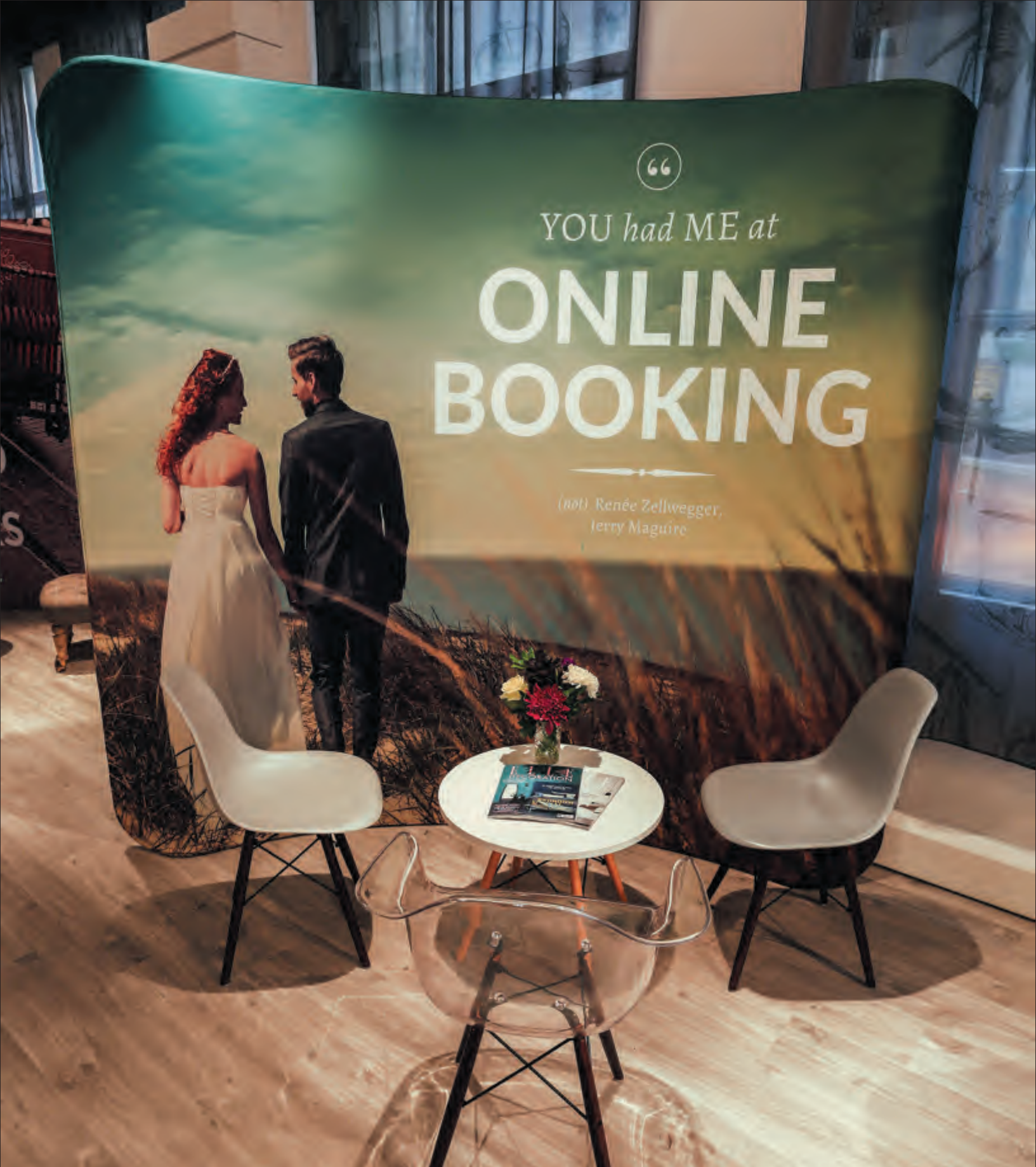
A Curve 24 ink-on-fabric display, inside Nettle of Birmingham Business Store. Each display comes in two parts – a lightweight aluminium frame, which clips together, and a fabric cover which stretches across the frame.
