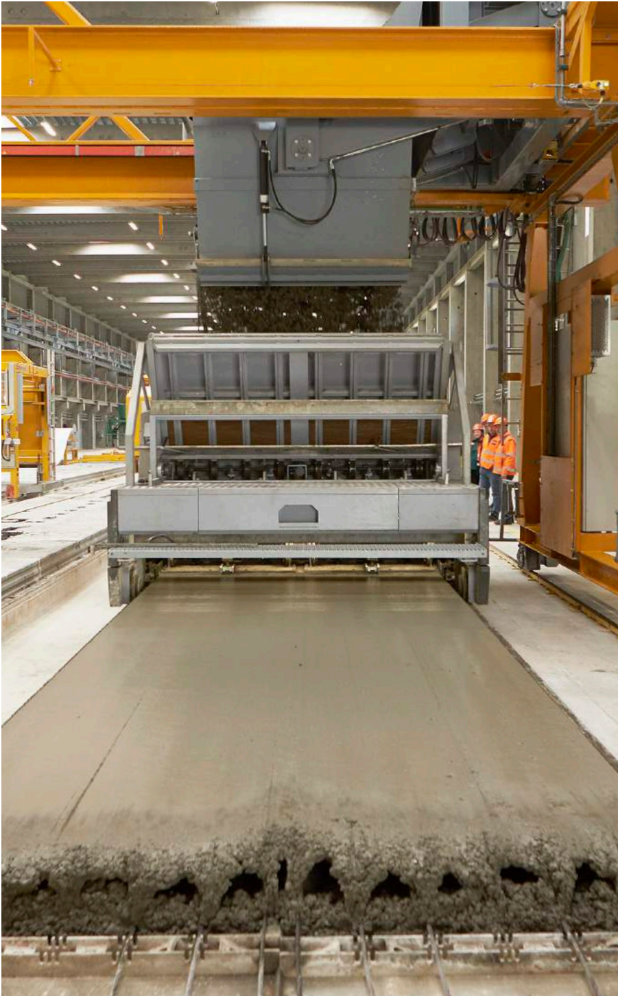
In 2018 CRH opened a new production hall at its hollow core plant near Copenhagen, Denmark, enabling it to meet growing customer demand for 240cm hollow core slabs and strengthening its position as the leading structural concrete producer in the country.
