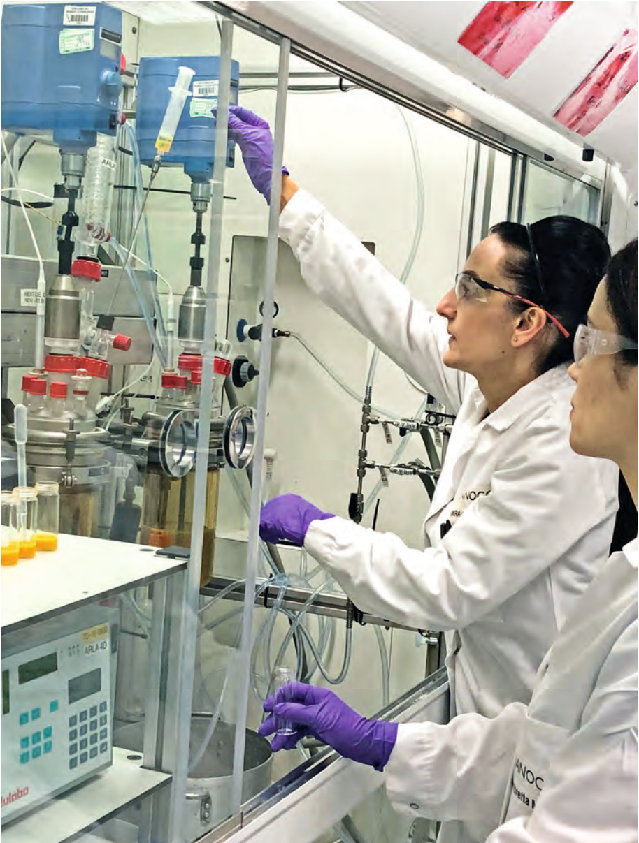
LEFT: Scale up chemists running small scale reactors for the production of CFQD® quantum dots.
