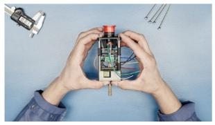
A Boeing 737 rudder trim switch is inspected.
