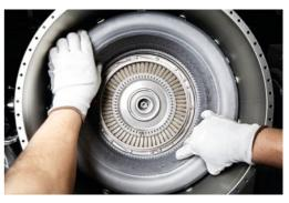
A PT6A engine is reassembled, inspected and tested before it is returned to service.
