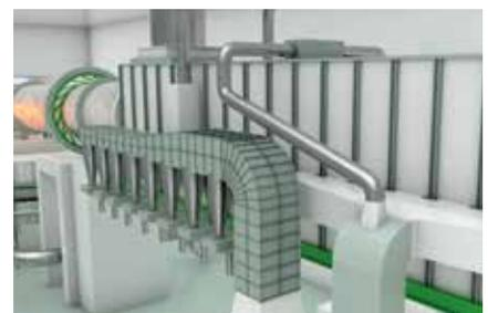
DRYING GREEN PELLETS IN TRAVELLING GRATE
