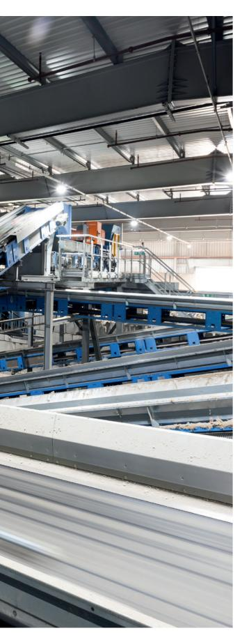
The purpose of the facility is to extract as much value from the waste it receives, by extracting the materials which have a value and can be resold. The residue is disposed of at a cost to a cement kiln, where it is used as fuel.
